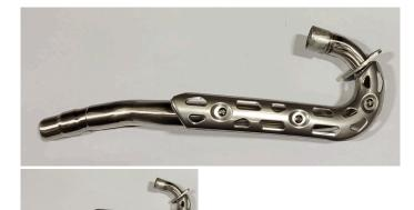
GX250 Parts GX250 Exhaust Pipe
